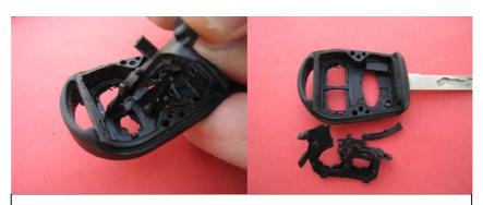
Once rubber starts parting from plastic cover, start pulling it gently and detach it. You should end up with cover looking like one in the picture above clean from old rubber remains
