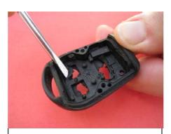
Use flat screwdriver to shave of old rubber layer. Do it gently so you do not damage hard shell.
