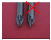
Do Not use Phillips screwdriver (shown on the right) as you may damage screws
