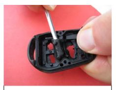
Continue rubber removing process using flat screwdriver with gentle shaving motion
