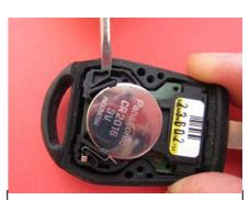
Gently lift electronic board to separate it from the top key part of the plastic cover
