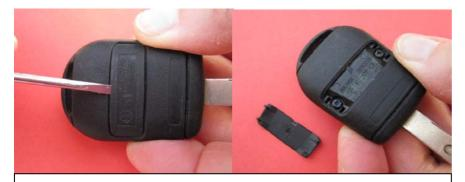
with flat screwdriver lift plastic cover positioned on the back of remote. You will uncover two screws which hold top and bottom part together
