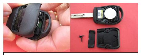
Lift back cover to uncover electronic board with immediately visible battery. After opening you will end up with parts as pictured above
