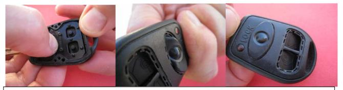
You have to push it in from inside the button using your thumb nail and manipulate it into position till whole button comes thru an opening.
