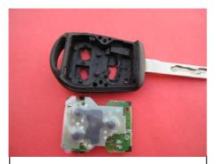
Separate electronic board with glued plastic protection cover. If clear cover is loose, re-glue it with super glue at the corners. Use very small dots of glue.
