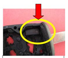
Important: please be careful not to damage Coding Chip located in the key part of the plastic cover at the bottom right corner
