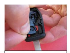
To fit new pad in you need to slide edge of oval button under the coding chip first.
