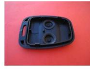
Top cover of remote with fitted from outside replacement buttons. (Internal view of the top cover)
