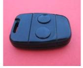
Closed Land Rover remote with fitted from outside replacement buttons
