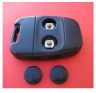
Land Rover remote after removal of an old rubber insert with embedded buttons
