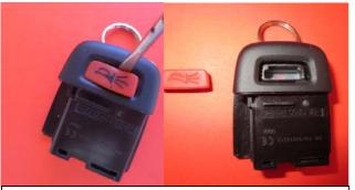
Depending on the condition of your button you can remove it simply by lifting up with flat screwdriver or with Stanley knife.
