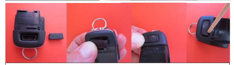
Next you press new Black panic button in using your thumb and finger nails. If it is bit hard to push with finger nails you can use blunt side of skewer to press on button edges.
