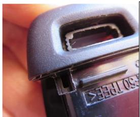
Before you start fitting new button in, make sure button cut out is clean from old rubber remnants.
