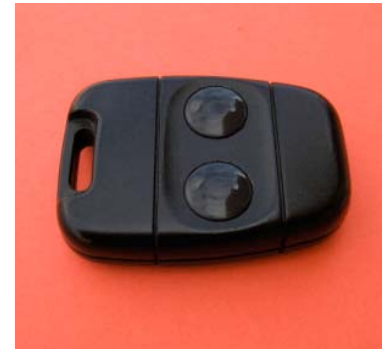
Closed Land Rover remote with fitted from outside replacement buttons
