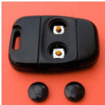
Land Rover remote after removal of an old rubber insert with embedded buttons
